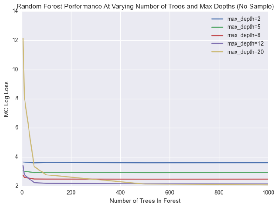
Figure 6: Random Forest (no sample) model performs better when more trees are in the ensemble. More complex base learners perform poor at smaller values of number of trees but quickly outperform the more simple base learners whose performance remains constant
