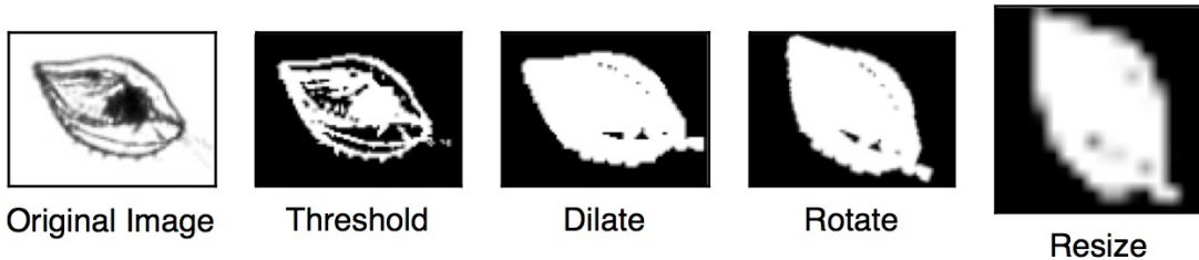
Figure 4: Series of mutations applied to each image to find the largest region and compare pixel by pixel features
